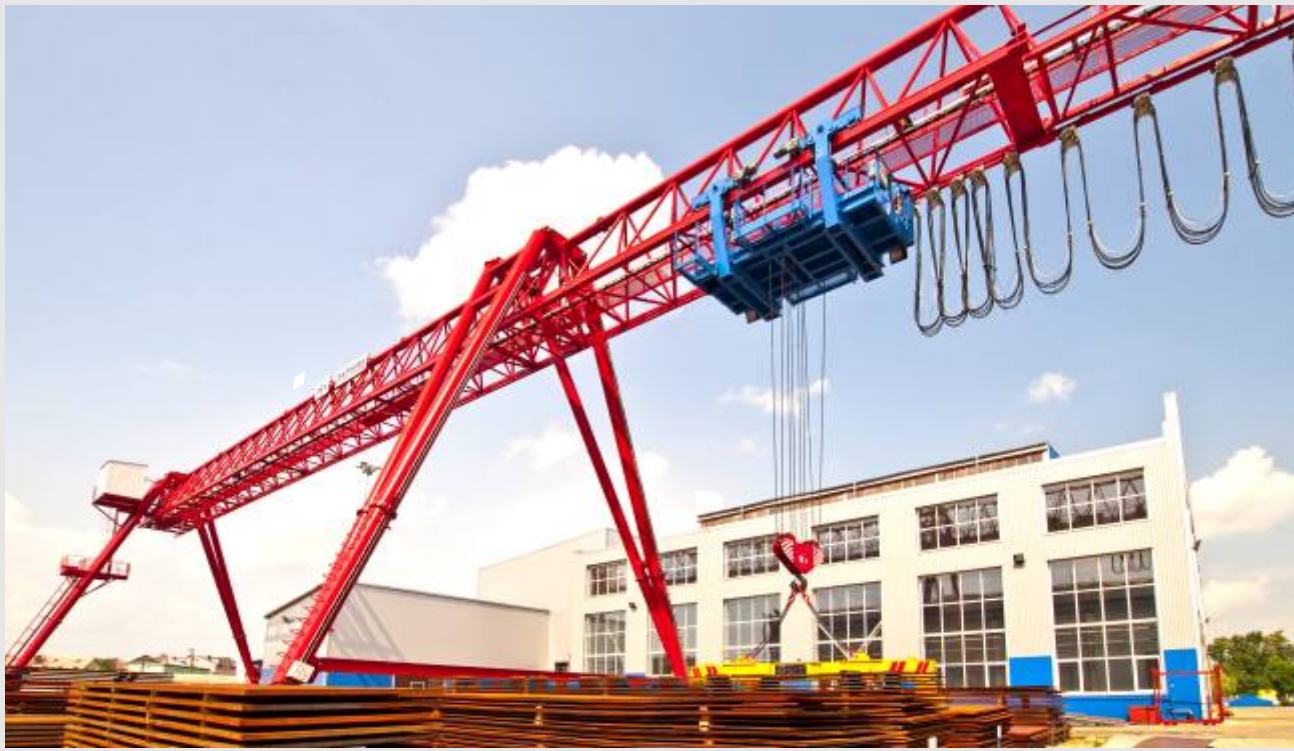
GANTRY CRANE WITH LATTICE TYPE BRIDGE
