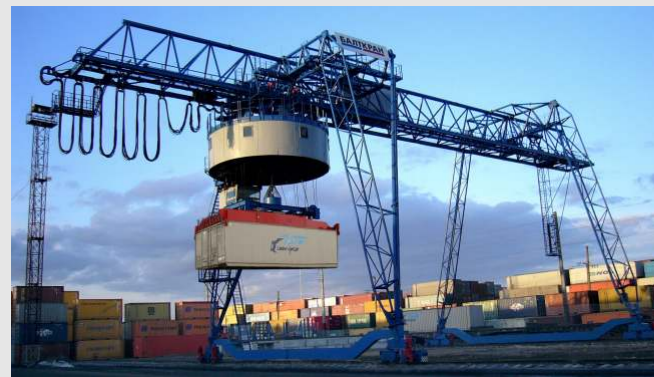
CONTAINER RAIL MOUNTED GANTRY CRANES
